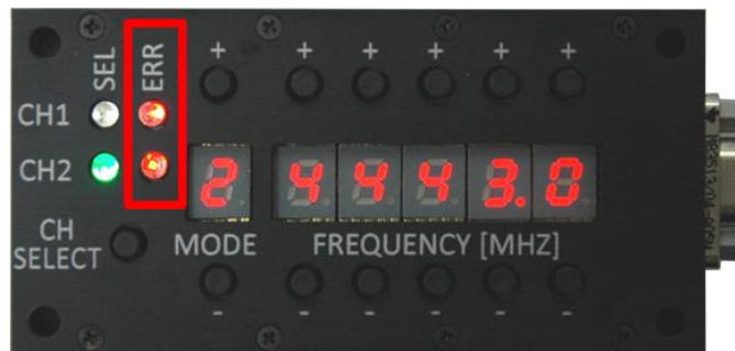
Figure 11: 2 nd Generation Switch Box Error LEDs, Two Blinking Red
