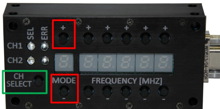
Figure 8: Increase LED Display Brightness Key Press Example
