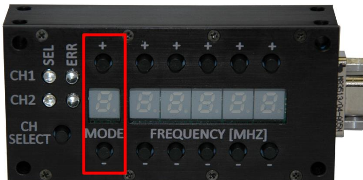
Figure 3: 2 nd Generation Switch Box Mode Selection
