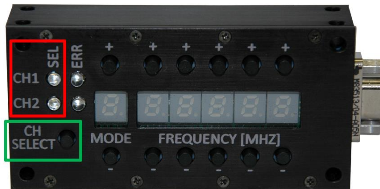
Figure 2: 2 nd Generation Switch Box Channel Selection
