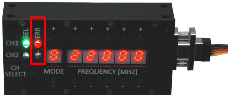
Figure 5: 2 nd Generation Switch Box Error LEDs
