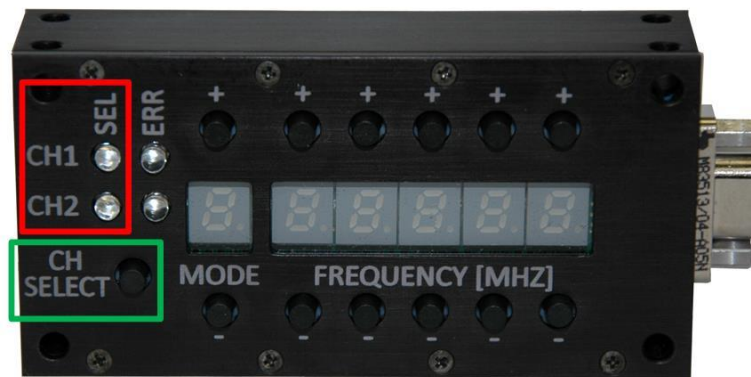
Figure 2: 2 nd Generation Switch Box Channel Selection
