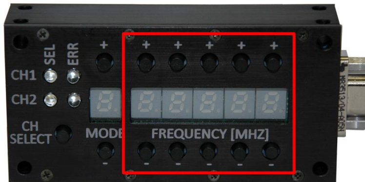
Figure 4: 2 nd Generation Switch Box Frequency Selection
