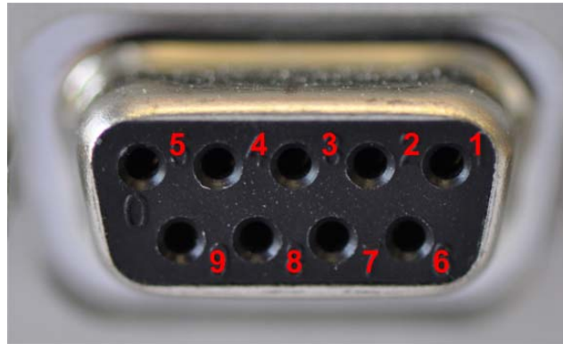
Figure 6: Front Panel DB-9 Serial Port Pins Labeled
