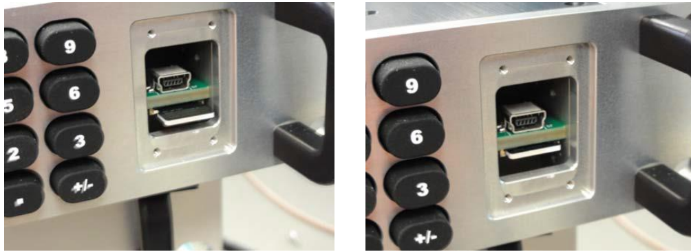
Figure 3: Micro SD Programming Card Inserted into Slot and Locked In
