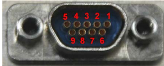
Figure 4: Female MDM-9 Connector
