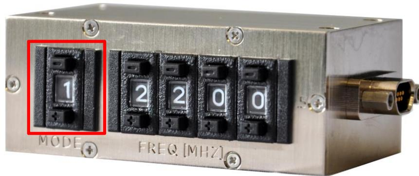
Figure 3: Front Close-up of Switch Box, Mode Digit Highlighted
