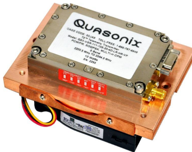
Figure 5: Bench Heat Sink shown with 6 cubic inch TIMTER™
