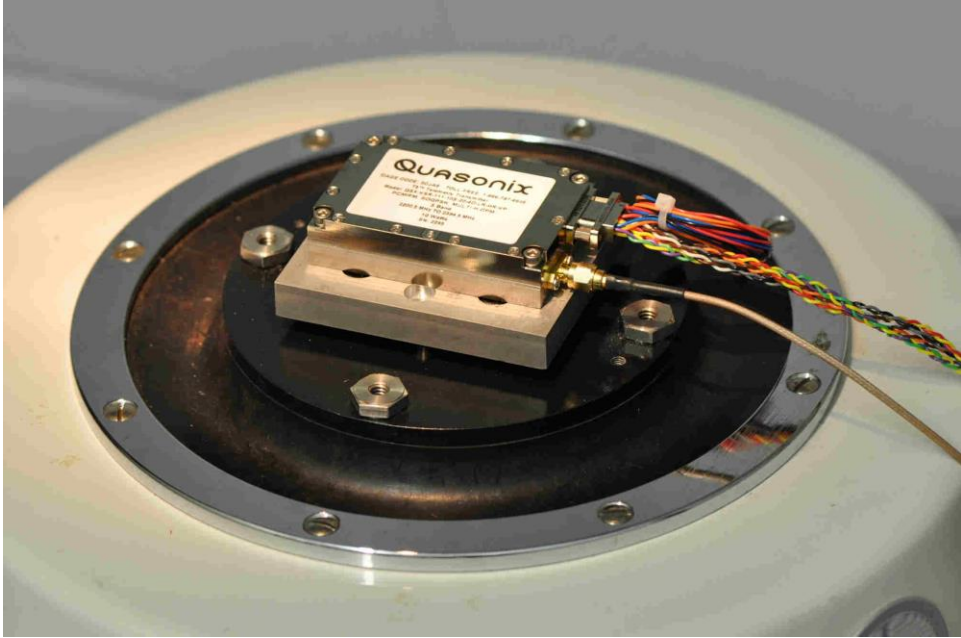
Figure 30: TIMTER™ Mounted for Z-axis Testing
