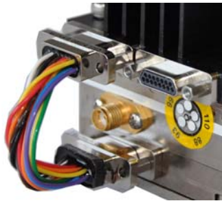
Connection to transmitter with a female MDM-15
