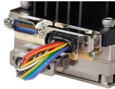
Connection to transmitter with a male MDM-15
